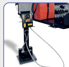
OPERATOR CONTROL CONSOLE Controls within easy reach of the operator
