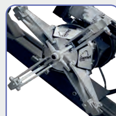
POWERFUL CHUCK For a secure grip on the wheel
