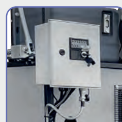
ELECTRICAL CABINET Integrated starter enclosure positioned at the front
