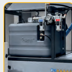
OIL TANK High-density polyethylene (HDPE)
